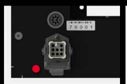
The new robust, moisture-proof **connection plugs** makes the electronic scoring target suitable for outdoor use.
