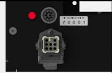
The **amphenol connector** offers direct connection option and various accessories such as printers.
